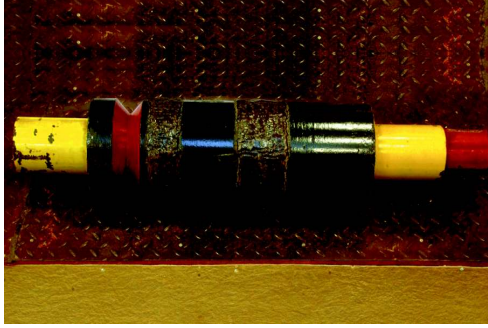
Shaft Keyway Crack
